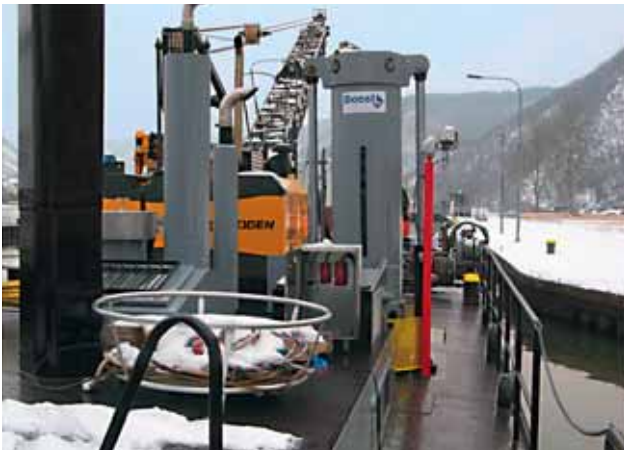
Armature cylinder of a dredger. The extension path of the telescopic device is detected with a VHZ of GHM.
