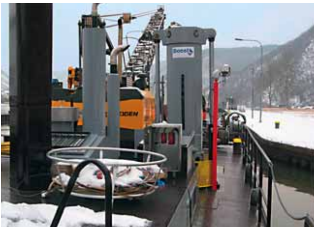
Armature cylinder of a dredger. The extension path of the telescopic device is detected with a VHZ of GHM.
