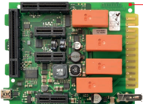
Relay card with 4 changeover contacts
